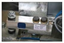
The features to be tested are detected by means of well-proven strain-gauge type load cells.
