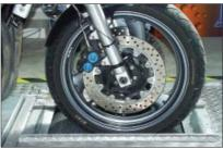
Car brake testers can be easily retrofitted for motorcycle tests.
